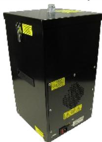
U-MARQ Super Swarf Extractor units have been developed for the safe and effective removal of swarf and smaller particles during processes such as routing, mechanical engraving, grinding etc. The pumps used in the U-MARQ Super Swarf Extractor are brushless and designed for continuous running with 30,000 hour use before servicing.
